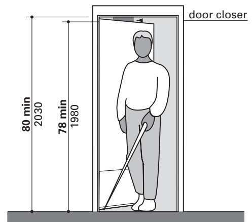
DR.26 Headroom and placement of a door closer or stop at a doorway or passageway
