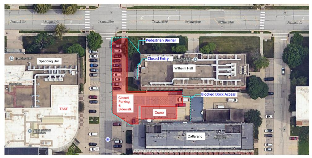
Wilhelm Hall HVAC Project. Two different crane mobilizations. The first crane will be on-site from April 23rd - <u>May 9th</u>. The second crane is tentatively-scheduled be on-site from May 21st - May 28th. Dock and tank access is limited, but can be coordinated in advance. Tanks can still be moved across the Wilhelm-Zaffarano dock during crane utilization.
